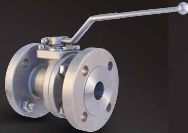
The 2-way Ball Valves with a floating ball are designed with a 2 or 3-part body. The floating ball design creates tightness on the downstream side, which keeps increasing as the up-stream pressure continues to rise.
