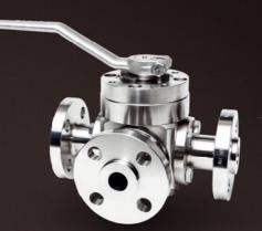
The 3-way Ball Valves with a floating ball are designed with a 2-component or multi-component body. The floating ball design creates tightness on the downstream side, increases as the up-stream pressure continues to rise. The valve is available with an L or T bore.
