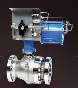
The 2-way Ball Valves with a floating ball are designed with a 2 or 3 piece body. The floating ball design creates tightness on the downstream side, which keeps increasing as the up-stream pressure continues to rise.
